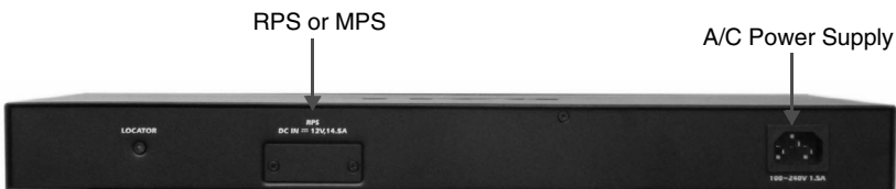
Figure 1-2. Back-Panel Power Connector
